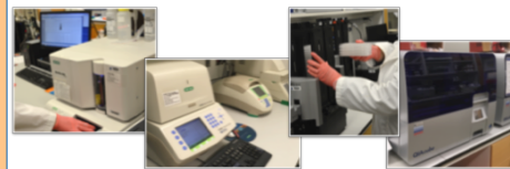
RBL Immunology supports research with specialized instrumentation including Luminex bead readers, quantitative RT thermocyclers, high-throughput multi-well plate washers/readers, and QIAcube sample preparation systems
